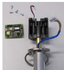
Remove board and board carrier. CAUTION: The board will be used again!
