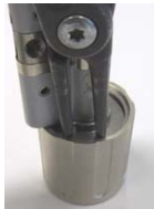
Loosen circlip ring with KESO circlip pliers and remove knob cover
