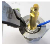
Remove circlip ring with KESO special pliers
